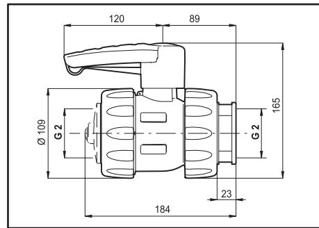
**Valvole a sfera con adattatore****Ball valves with cam-lock male adapter****Válvulas de bola con adaptador macho**
